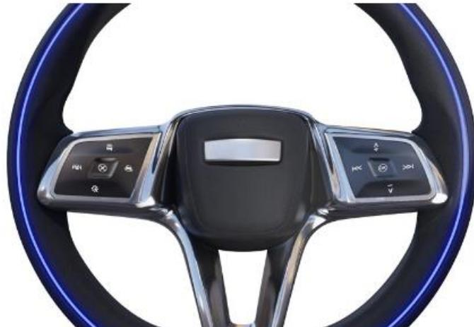
The 3D-printed composite airbag housing container prototype housing within a full steering wheel.
