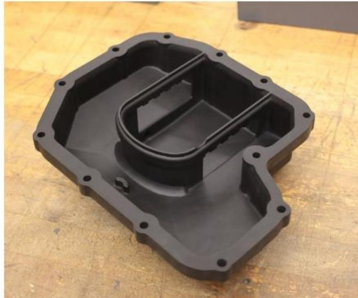
This 3D-printed composite oil pan was built using Windform SP material for the University of Victoria's 2019 SAE racecar. Source | CRP Technology
