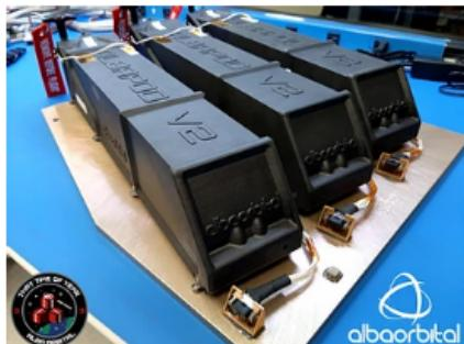
Alba Orbital will take customer satellites to orbit on a SpaceX Falcon 9 launch vehicle in December 2020 as part of a rideshare agreement. It will be used the company's AlbaPod v2, the world's only space proven PocketQube deployer. It has been entirely 3D printed by Italy-based CRP Technology using their Windform XT 2.0 high-performance composite material Carbon-fiber reinforced from Windform TOP-LINE family of composite materials.
