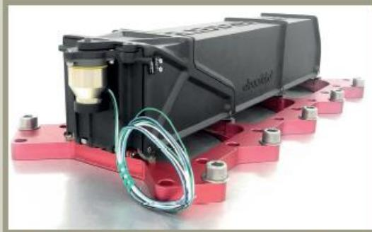
Fig.1: 3D printed AlbaPod 2.0 on vibration table going through preflight certification
