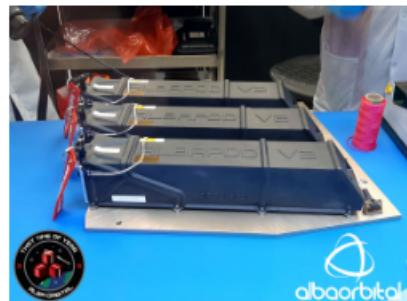
Recently Alba Orbital's AlbaPod V2 hyped up for its unique design, lightweight, easily integration into space launch vehicles, maintenance of the demanding quality standards for space. These characteristics have also made possible thanks to the use of AM and Windform XT 2.0 Carbon composite material
