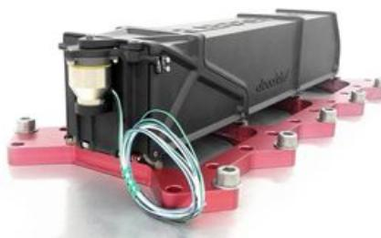
The 3D printed AlbaPod 2.0 on a vibration table going through preflight certification. (Photo courtesy Alba Orbital.)
