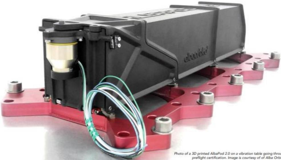
Photo of a 3D printed AlbaPod 2.0 on a vibration table going through preflight certification. Image is courtesy of Alba Orbital.
