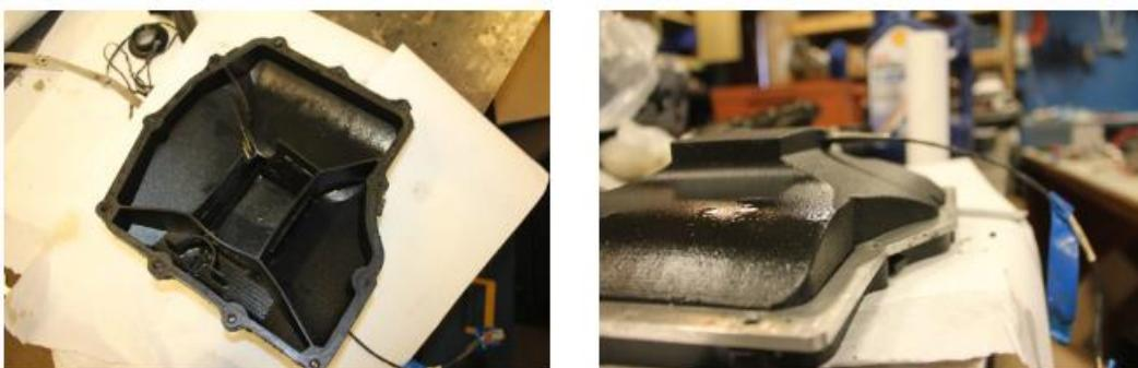
The oil pans for the 2016, 2017 and 2018 vehicle were printed using Carbon-composite material Windform® XT 2.0.
