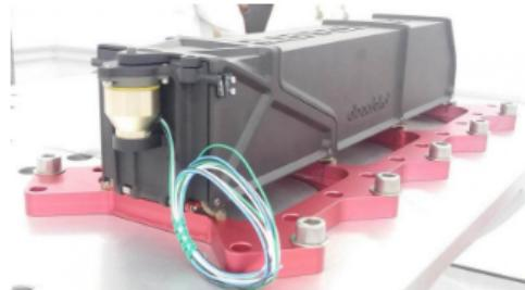
3D printed AlbaPod 2.0 on Vibration table going through preflight certification. Courtesy Alba Orbital
