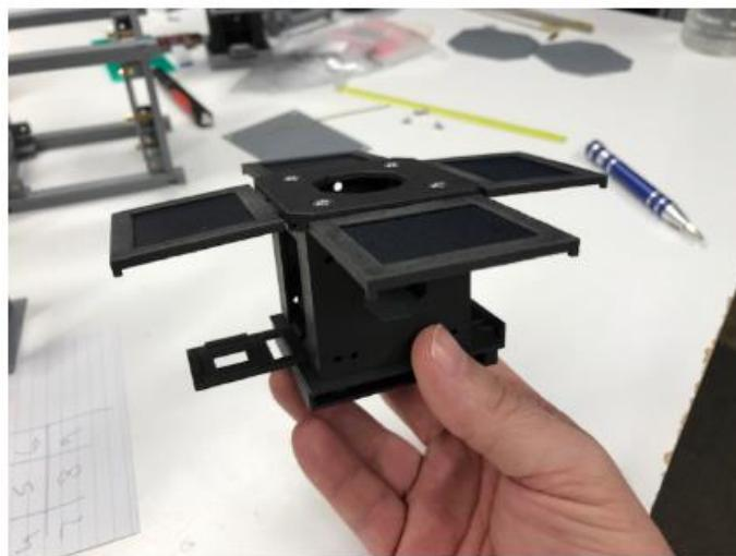
First assembly of the Windform Frame. Photo via Mini-Cubes.
